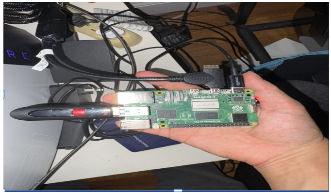
Fig. 4. Our edge device (Raspberry Pi) with an attempt to run a quantized model.
